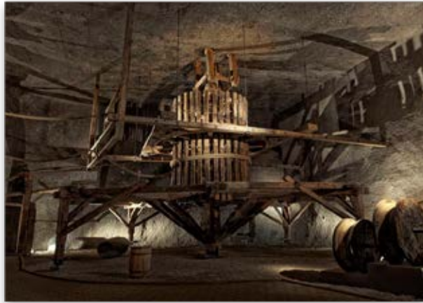
A wooden hoisting machine, 18th century (a Hungarian-type)
